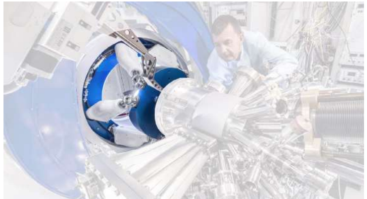
Diffractometer with BREVA hexapod on CEA BM32 beamline at ESRF synchrotron for the development and analysis of nanomaterials.
