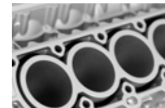
Nikasil® layers in aluminum cylinders
