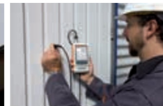
Measurement of a paint coating on steel
