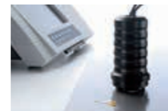
Hand probe with beta emitter
