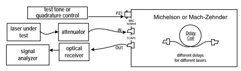
Laser under test is input to interferometer, which is set to the appropriate optical path mismatch by selection of the delay line which may be user installed or changed. Voltage control is applied to the PZ1 fiber stretcher input to maintain quadrature bias. Output optical signal is applied to an optical receiver. Receiver output to a signal analyzer or digitizer / recorder.
