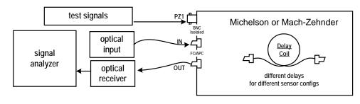
Optical input applied to represent the optical source of a fiber interferometric sensor. Delay coil is selected to be length of sensor to be simulated. Test signals applied to the PZ1 fiber stretcher. Output optical signal is applied to an optical receiver. Receiver output to a signal analyzer or digitizer / recorder.
