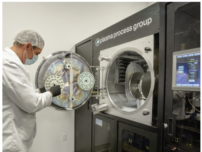
Ion Beam Sputtering (IBS) Chamber for Ultrafast Optics at Thorlabs' Headquarters in Newton, NJ
