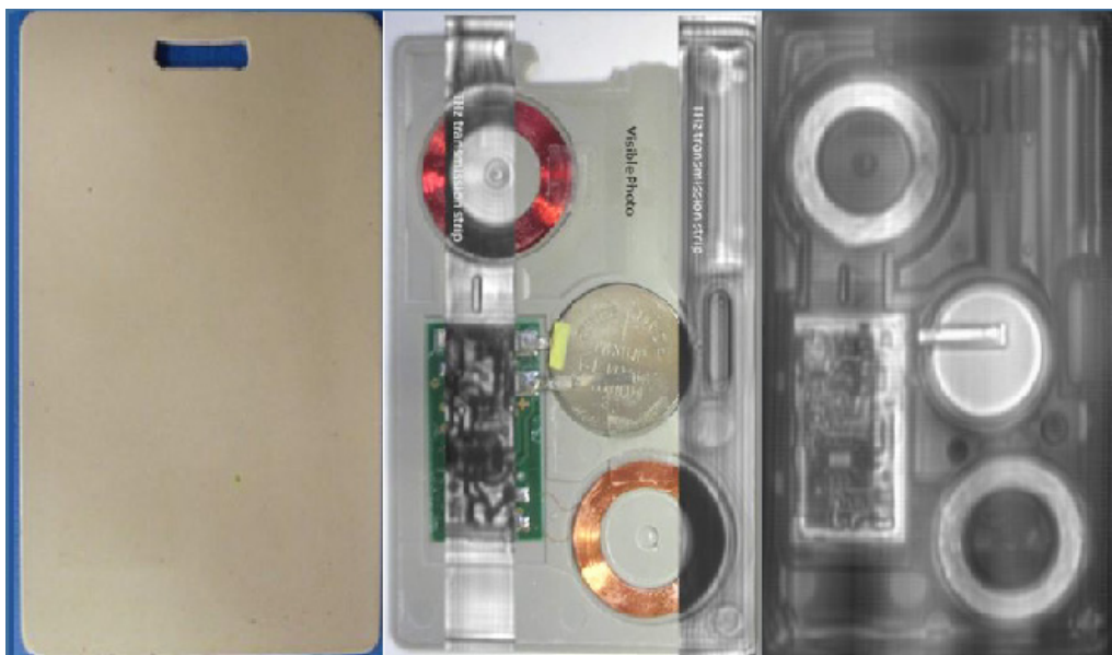
Visible image of opened card with THz transmission strips
