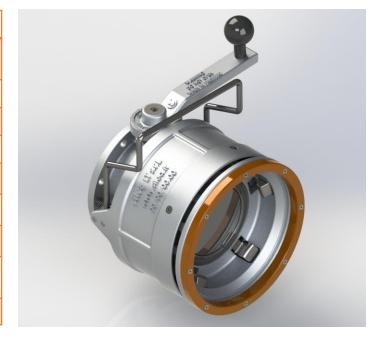
The main component of the oupler are made in aluminium alloy. Standard seals in fluoroelastomer FKM-GLT (Viton® for -40°c/+200°c) are easy to maintain. The surfaces subject to wear are hard coated.
