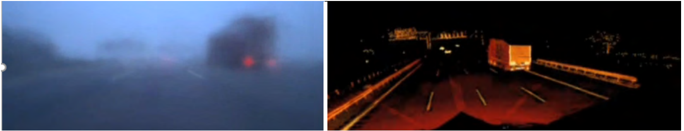
Figure 8: Camera vs. LiDAR in mist/rain
