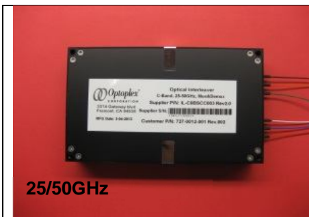
Figure 31 - 25/50GHz Mux/DeMux Co-Packaged Interleaver Module.
