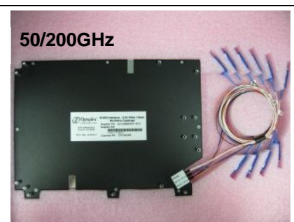
Figure 33 - 50/200GHz Two-Stage Mux/DeMux Co-Packaged Interleaver Module.
